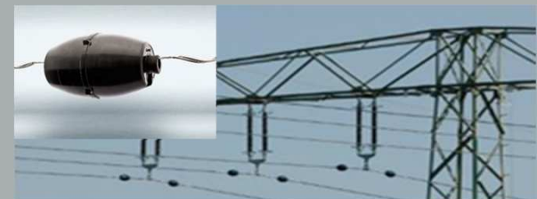
Industrial: Autarkic sensors for power line monitoring
