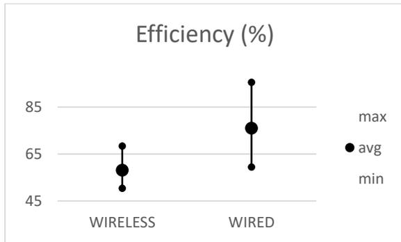
Figure 3 - Charger efficiency span
