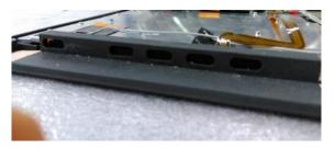
Fig. 15. Frame prototype 3D printed in plastics – connectors' slots view
