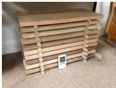
Fig. 13. Climatizing timber prior to machining
